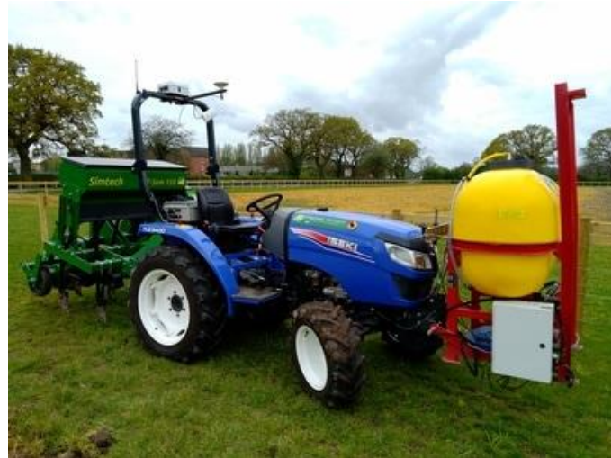
Figure 3 – Modified Iseki tractor of the Hands Free Hectare project [57].
