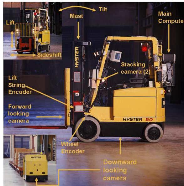
Figure 5 – Tug and forklift used for experimental purposes in [72].
