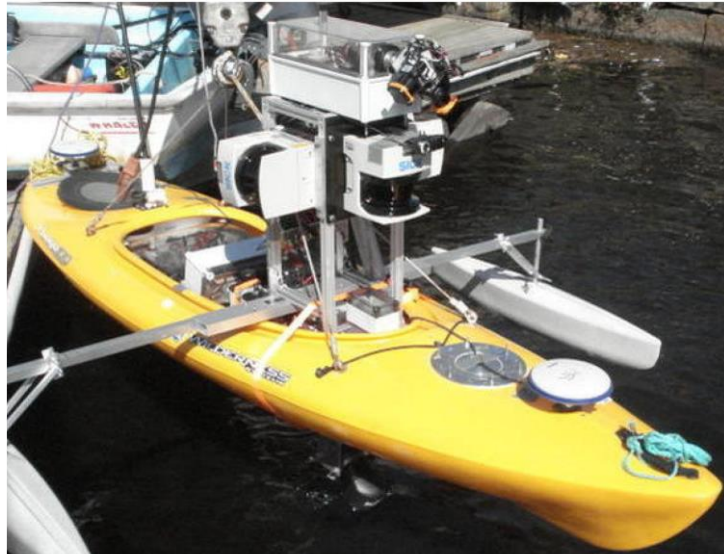
Figure 9 – ASV based on SCOUT robotic kayak with additional sensors employed in [96].
