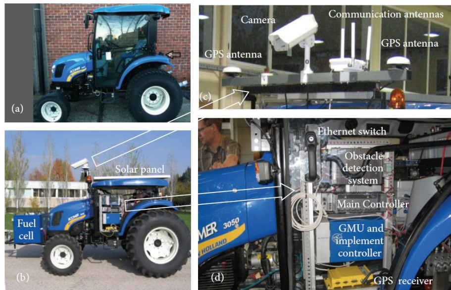
Figure 2 - (a) Original CNH Boomer-3050 tractor, (b) modified RHEA vehicle, (c) external equipment on-board the mobile units, and (d) internal equipment distribution inside the mobile unit's cabin [28].
